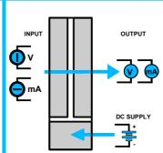
Isolated converter for voltage and current configurable by **Dip-Switch or PC**
