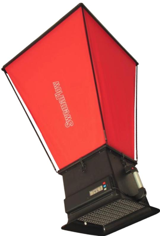
**SwemaFlow 4001** is ideal for testing, adjusting and balancing (TAB) of air flows up to 1500l/s , 3100cfm. SwemaFlow 4001 uses the proven Swema principle, a net of hot wires, which gives a good and accurate mean value for supply and exhaust air flows. Measured values can be stored and transferred to PC.
