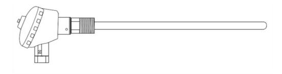
Chart 2: A tube thermocouple with a cable
