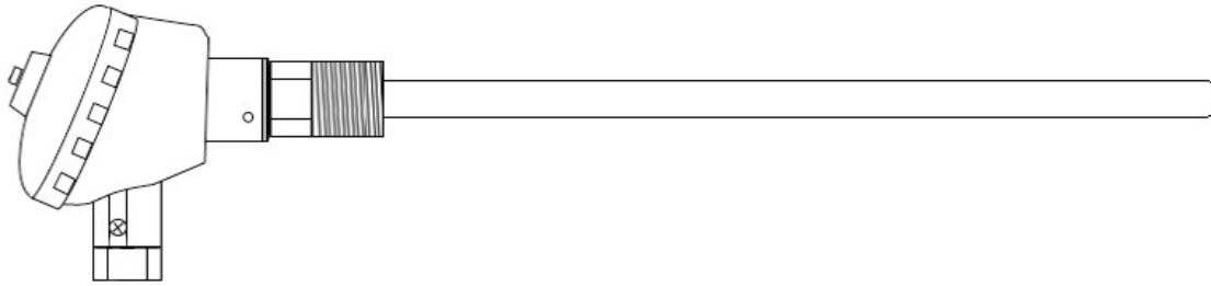
Chart 1: Industrial thermocouple with an either ceramic or SS 316 tube
